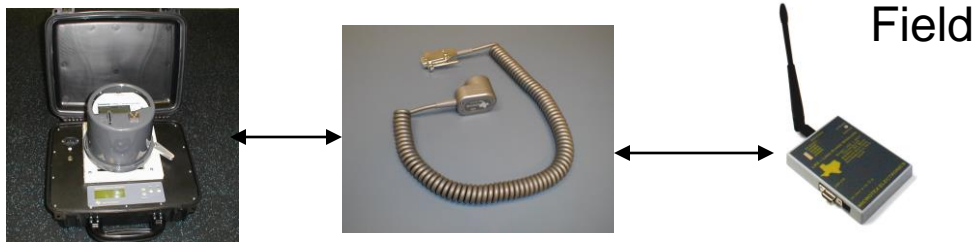
Metertest-1 with Optical probe and LR2 Wireless
